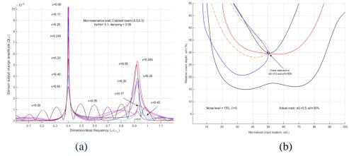
Fig. 3. Measured sensor output charge (a) and diagram for crack detection (b)
