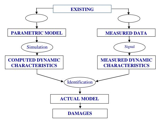
Fig. 1. Flowchart of damage detection process
