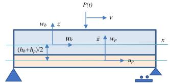
Fig. 2. Model of beam structure bonded with a piezoelectric layer under moving load
