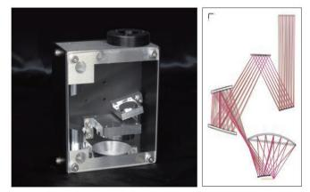
(Designed for focusing and irradiation of femtosecond-laser pulses)
